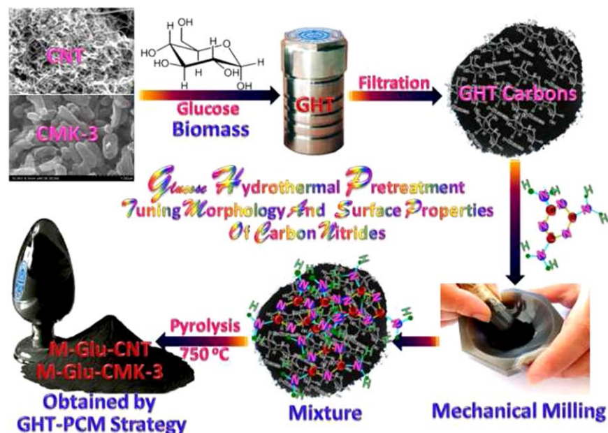
Scheme 1. Illustration of synthetic procedure for novel carbon nitride materials with tunable microstructure and surface chemical properties (M-Glu-CNT or M-Glu-CMK-3) through a facile and scalable mechanical milling and subsequent pyrolysis approach of the glucose hydrothermally pretreated carbonaceous materials like CNT or CMK-3 with melamine.
